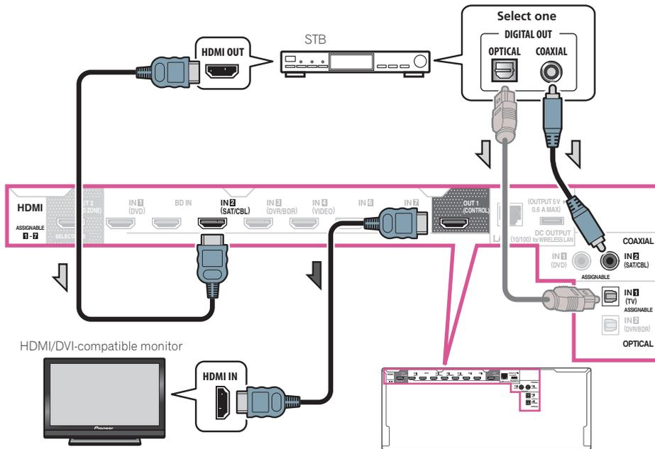
— If you use a digital audio cable or RCA (analog) audio cable, you'll need to tell the receiver which digital input you connected the set-top box to (see [The Input Setup menu](#) on [page 40](#)).
