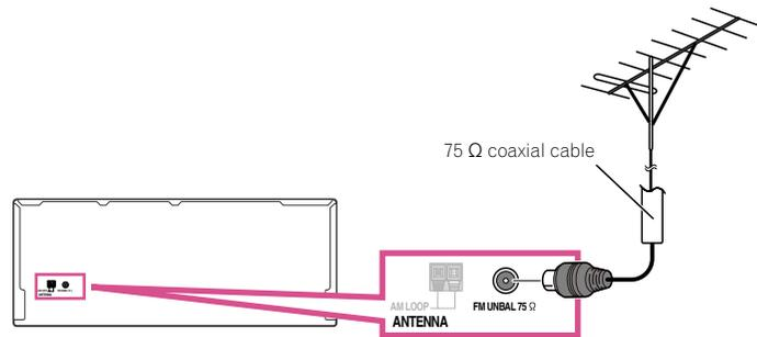
To improve AM reception, connect a 5 m to 6 m (16 ft. to 20 ft.) length of vinyl-coated wire to the **AM LOOP** terminals without disconnecting the supplied AM loop antenna. For the best possible reception, suspend horizontally outdoors.
