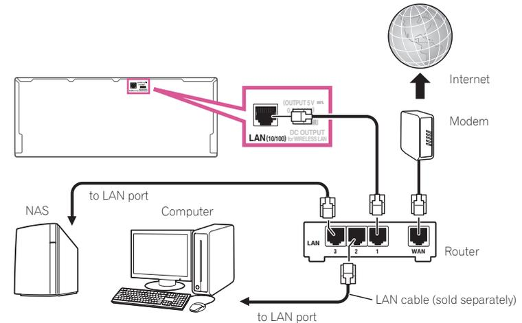
Connect the LAN terminal on this receiver to the LAN terminal on your router (with or without the built-in DHCP server function) with a straight LAN cable (CAT 5 or higher). Turn on the DHCP server function of your router. In case your router does not have the built-in DHCP server function, it is necessary to set up the network manually. For details, see [Network Setup menu](#) on [page 90](#).
